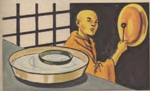
In the Chinese and Indian waterclocks a small brass bowl with its bottom pierced was floated on a basin of water. The floating bowl gradually filled with water, and, after a measured interval of time, sank. An attendant then struck a gong and set the bowl afloat again.
